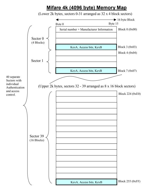
The lower 2048 bytes of the 4k card (sectors 0 - 31) are organised in the same way as the 1k card. However the upper 2048 bytes are organised as eight large sectors of 16 blocks each (sectors 32 - 39). Taking into account the Serial Number/Manufacturers Block and the Sector Trailer Blocks then there are 3440 bytes of free memory for user storage.
