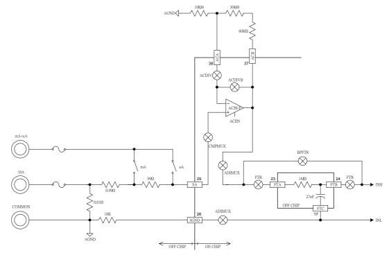
Graph 21. Function network diagram of DC current.
