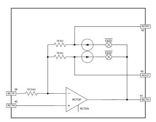
Graph 7. Full-wave rectifier switch block
