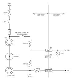
Graph 25. Function network of diode measurement.
