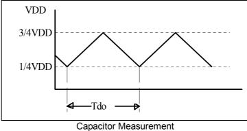
To calculate the cycle, we send the square wave that out from CAPTG to the frequency counter. When operating the frequency measurement, the necessary timer reference signal is FTB. For the measuring frequency, it can be gained through the following formula. In this formula, Ksg is the signal counter and Ktb is the value of the time-base counter.
