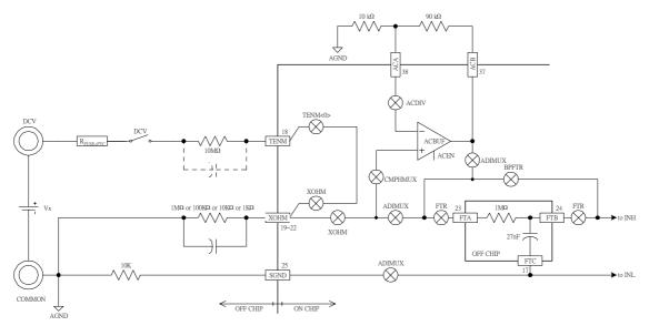
Graph 19. Function network diagram of DC voltage.
