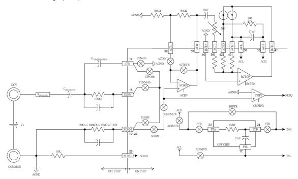
Graph 20. Function network diagram of AC voltage.
