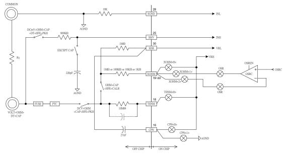
Graph 23. Function network diagram of resistor.
