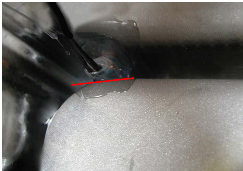
Illustration 8.5.1 Position and silicone fixation of overheating
