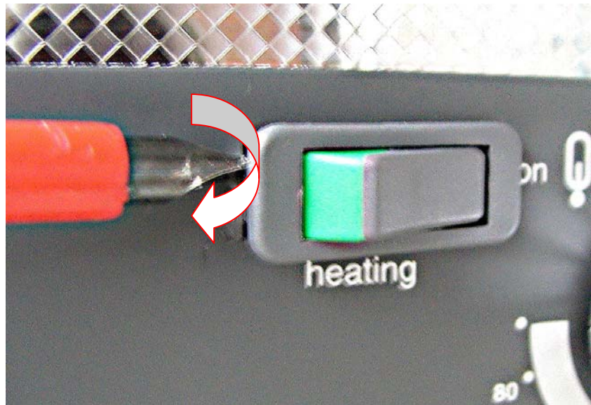
Illustration 8.3.3. Levering the heating switch out of the front plate
