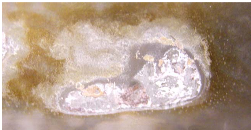
Illustration 9.1. Lime deposits due to insufficient stirring
