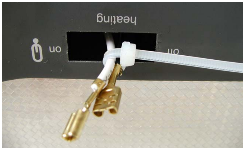
Illustration 8.3.4. Secure the cables
