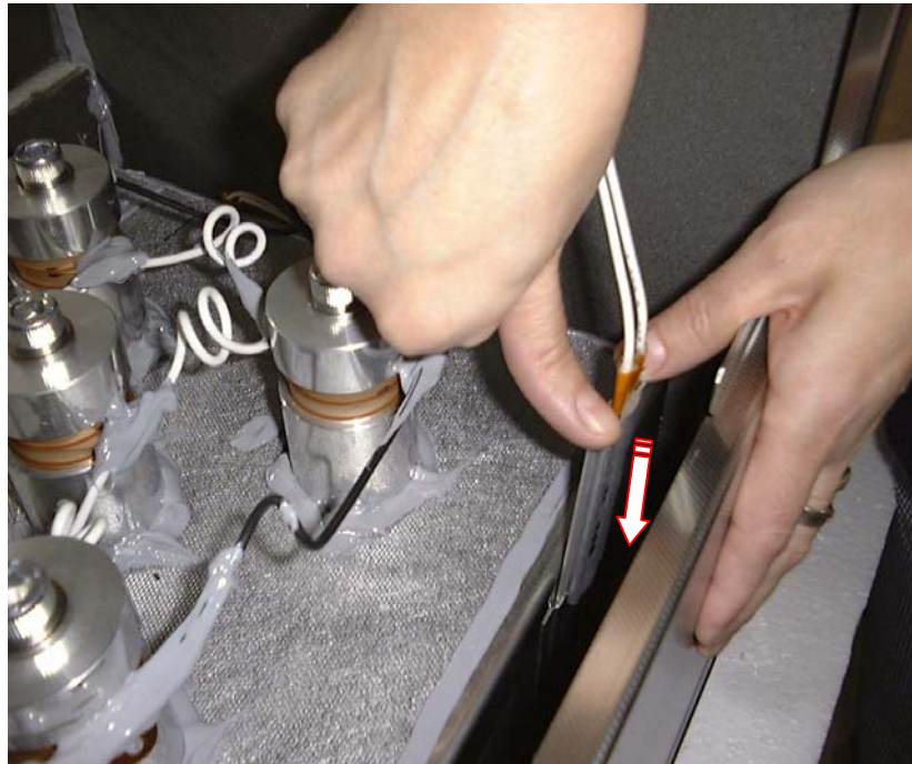
Illustration 9.4. Mounted tank with vertically fixed heating elements. Push the new heating element(s) into the guiding rails into the marked direction.
