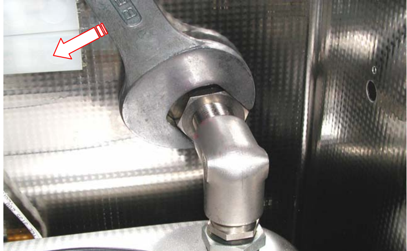
Illustration 12.1.4. Loosen the lock nut with a 32 mm fork wrench anti-clockwise
