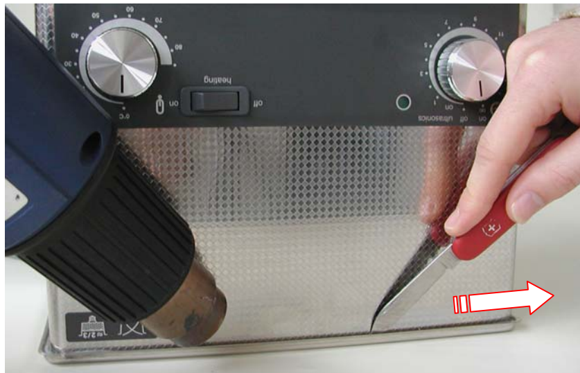
Illustration 11.1.1. Heat up the silicone sealing in the tank edge and cut with a knife.
