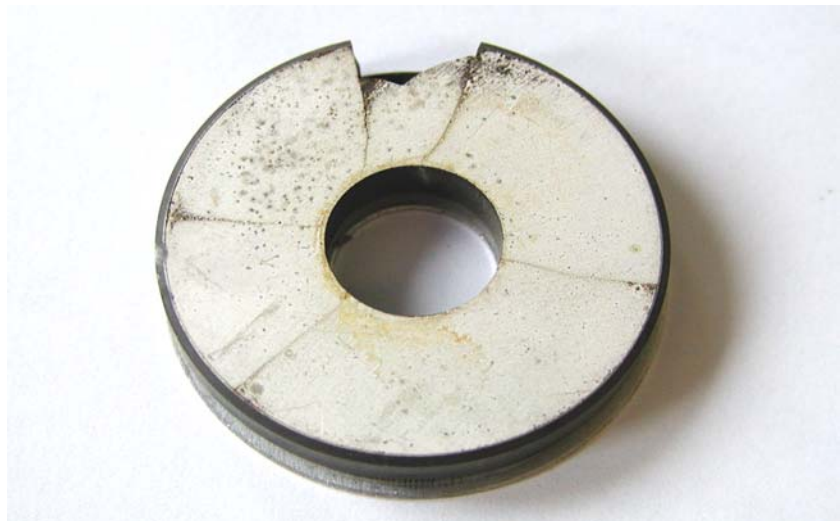
Illustration 10.1. Torn and broken PXE transducer disk
