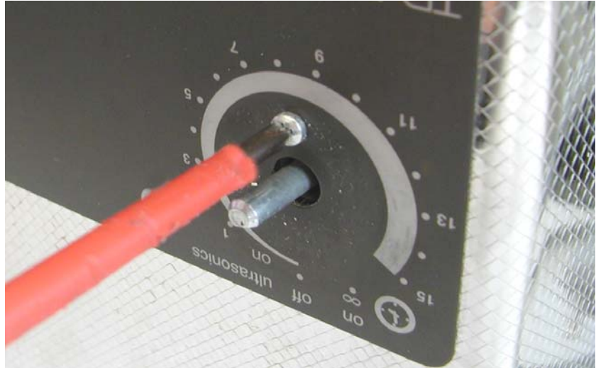
Illustration 7.1.1. Remove the recessed head screw (under the turning knob)
