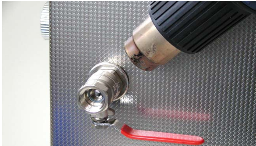
Illustration 12.1.5. Heat the Loctite thread sealing with a hot air fan
