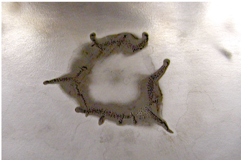
Illustration 11.1. Heavy cavitation erosion at the spot where the transducer system is fixed
