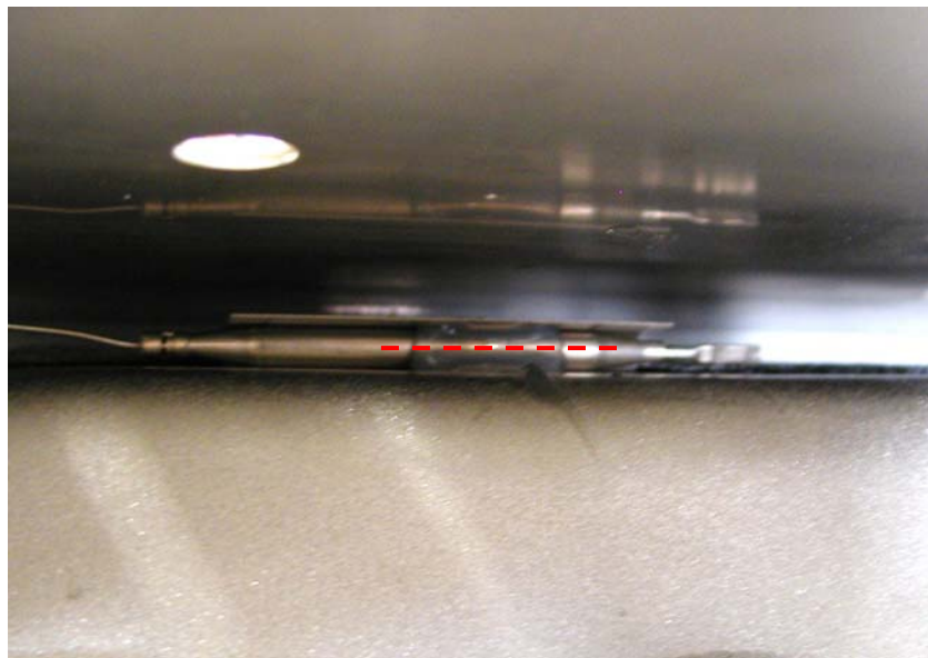
Illustration 8.6.2. Capillary probe clamped-in and secured with silicone (since Feb 2002) red dotted line: cut silicone here to remove the probe
