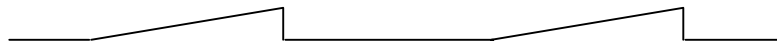
Illustration 16.2.4.: Current graph in case of short circuit in output transformer or transducer system
