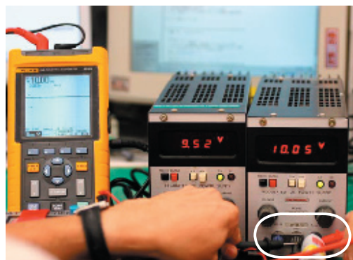
Measure the voltage between the electrode sections (+ and -).
