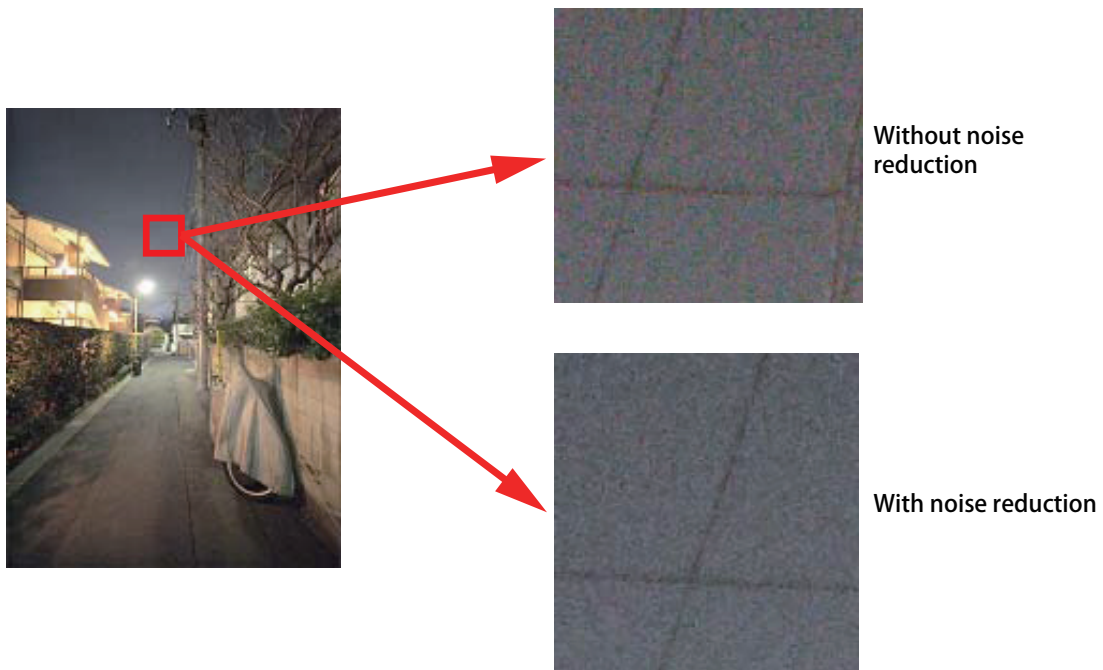
Fig. 005 Sample images comparing the effect of chrominance noise reduction
