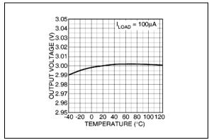
*FIGURE 2-14:* Output Voltage vs. *Temperature.*
