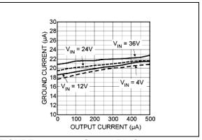
FIGURE 2-6: Ground Pin Current vs. Output Current.
