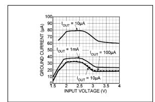
*FIGURE 2-10:* Ground Pin Current vs. Input Voltage.
