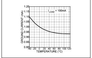
**FIGURE 2-9:** Ground Pin Current vs. Temperature.
