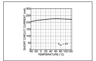
FIGURE 2-15:Short-Circuit Current vs.Temperature.
