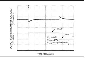
FIGURE 2-16: Load Transient Response.
