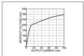
FIGURE 2-2: Dropout Voltage vs. Output Current.
