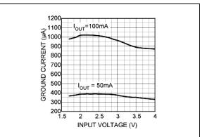
FIGURE 2-11: Ground Pin Current vs. Input Voltage.
