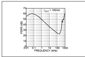
FIGURE 2-1: Power Supply Rejection Ratio.
