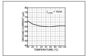
**FIGURE 2-7:** Ground Pin Current vs. Temperature.
