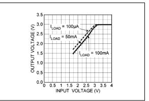
FIGURE 2-4: Dropout Characteristics.
