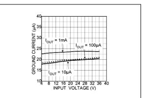
FIGURE 2-12: Ground Pin Current vs. Input Voltage.
