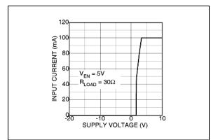
FIGURE 2-13: Input Current vs. Supply Voltage.
