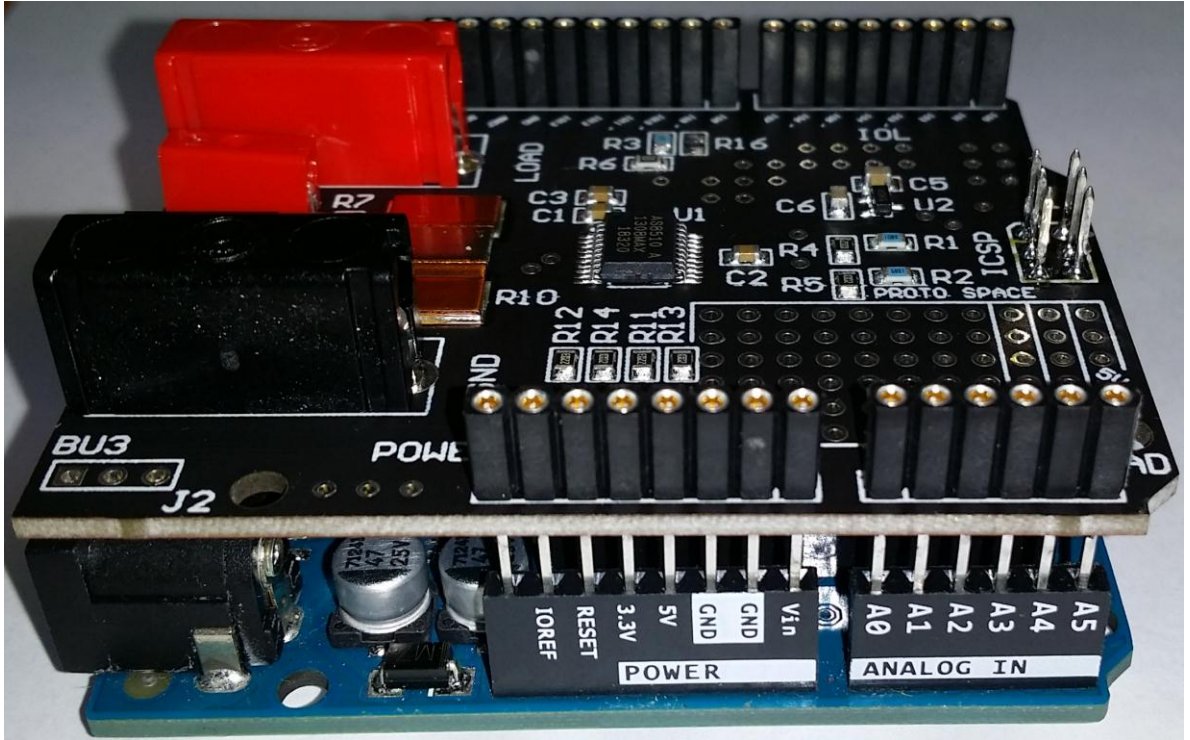
Figure 2: AS8510 Arduino Shield connected to the Arduino Uno board
