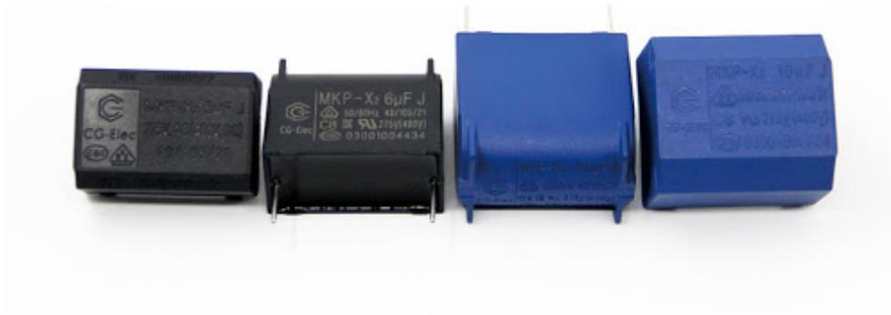
Figure8. Filter Capacitors
