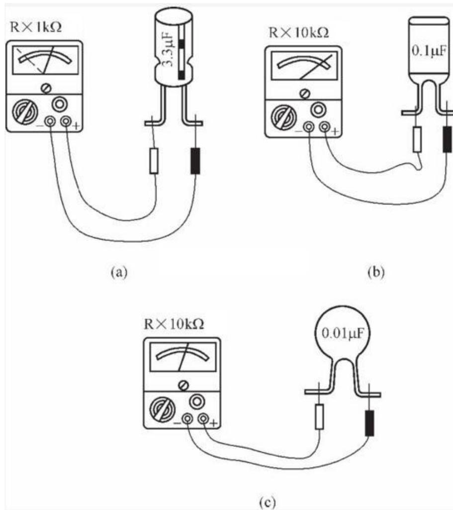
Figure12. (a) Normal; (b) Breakdown; (c) Failure
