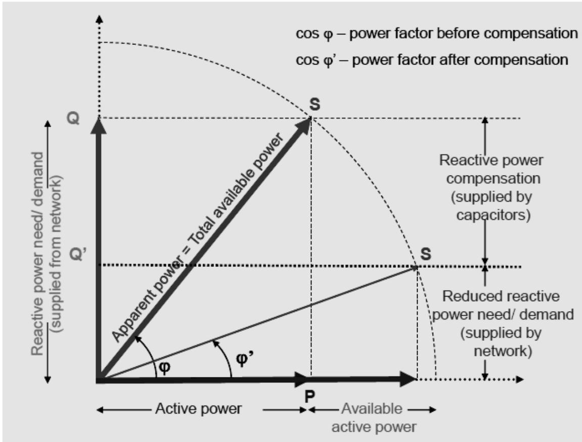
Figure 11. Reactive Power Compensation Supplied by Capacitors
