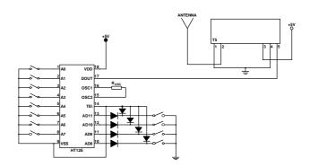
**Figure 3: RS-MK Transmitter Application Circuit**
