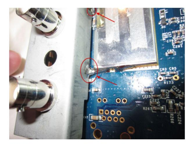
Also Your soldering station should have enough power to warm up the metal, otherwise the connection will not be reliable.
