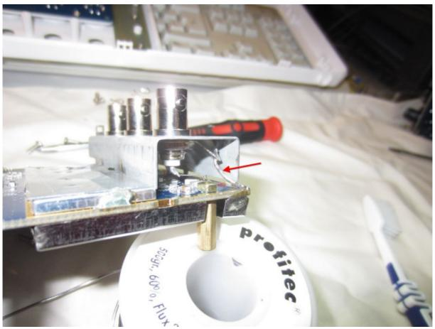
The next point is the BNC ground connection which is not optimal for HF purposes. I bend down the soldering strap of the channel 1 BNC for it is the only one which is simply reachable. Then I took 1mm copper wire and soldered it on the pcb ground and the strap.
