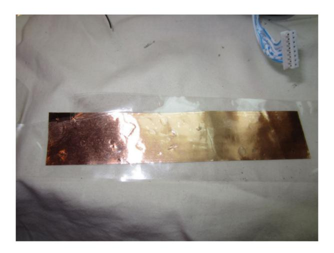
For the ground connection we have to solder a wire in one of the corners. After that we wrap the shielding around the VGA wire. The GND wire must be near the VGA out connector. I tied around the shield some stripes of tape to avoid later opening of the shield.
