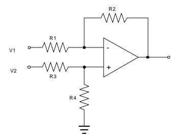
Let's apply the principal of superposition to the Differential Amplifier. The Differential Amplifier uses matched resistors to give us a single-ended output that is the result of the difference in voltage between V1 and V2. If we ground V2, then we have the basic inverting amplifier and  $Vout = -\frac{R_2}{R_1}V_1$ . If we ground V1, then we have the basic non-inverting amplifier except that the +IN voltage is a divided version of V2.
