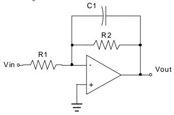
The transfer equation is the same as we derived earlier for the inverting amplifier, except that now we have the parallel combination of C1 and R2 in place of R2. The impedance of the feedback network is:
