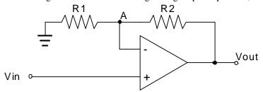
This circuit still has negative feedback so we can apply our two rules. Node A will be equal to the input voltage. The current in R1 is equal to  $\frac{Vin}{R1}$  and the current in R2 will be  $\frac{(Vout-Vin)}{R2}$ . Now since those
