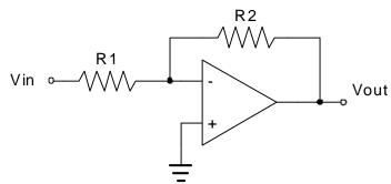
From rule 1 we know that both inputs are at zero volts. And from rule 2 we know that any current which flows in R1 must also flow in R2 since rule 2 specifies that no current flows into the (-) input. Now we can write an algebraic equation and solve for the response of this circuit.
