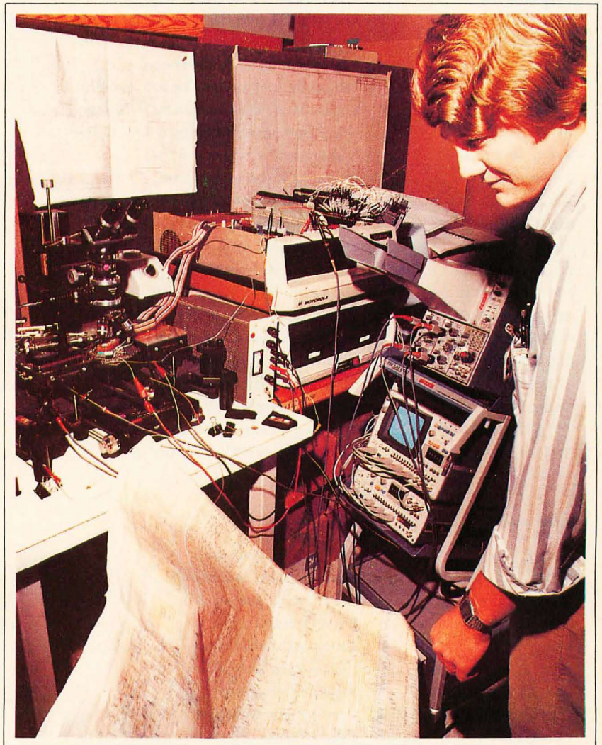
Photo 5: First silicon engineering analysis. Logic and circuit design engineer Bob Thompson tracks down a weak node in the first batch of 6801 chips. The 6801 die is packaged, but not sealed, so that internal nodes may be probed while in operation. Viewing through the microscope, a probe can be placed at critical points equivalent to the layout plot. The chip itself is running a modified EXORcisor system, and the scope actually displayed an internal signal with excessively slow rise time.
