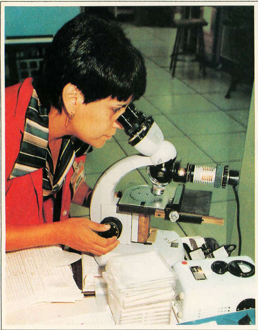
Photo 3: Visual inspection. Some of the gross processing errors or problems that occur with probing equipment can be detected visually. Here, lead production operator Mary Celedon checks a 6802 wafer.
